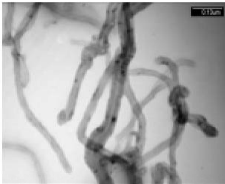
Fig.1 TEM image of purified MWNTs
